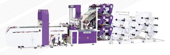
BJAF+S No Tension Type Servo Control Heavy Duty Bag Making Machine
